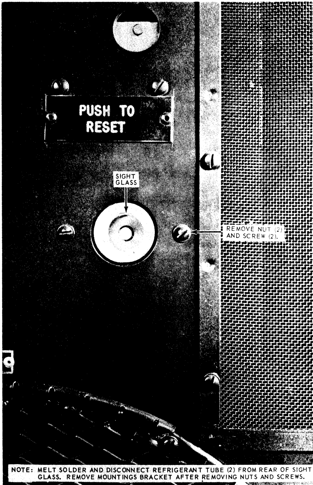
Figure 5-7. Sight glass, removal and installation.
